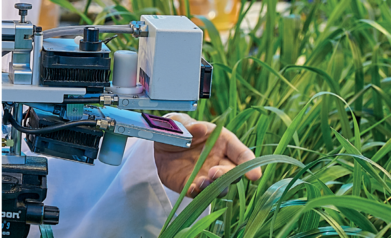
An IAPN scientist choosing the newest fully expanded leaf in a wheat plant in order to measure the leaf gas exchange. (Photo: K+S)
