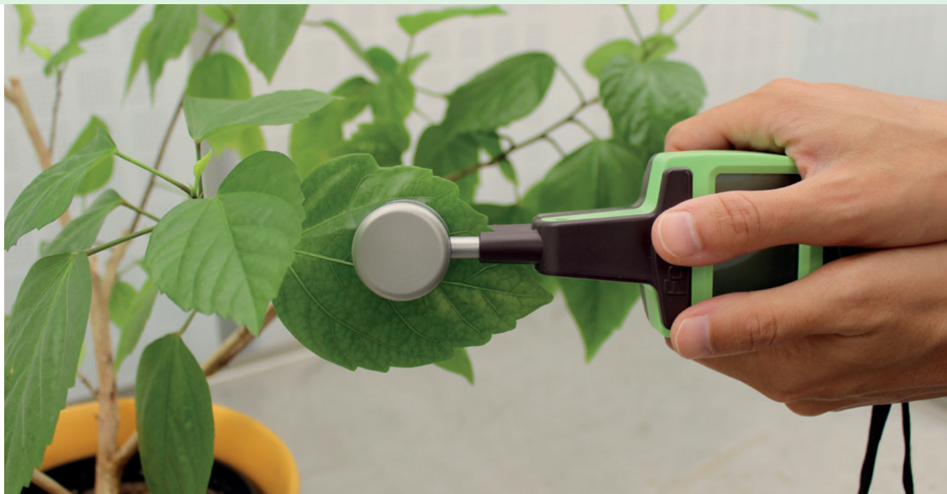
Assessing the pigment content in leaves, using the optical sensor Dualex, allowing real time results with non-destructive means. (Photo: Jamali Jaghdani)
