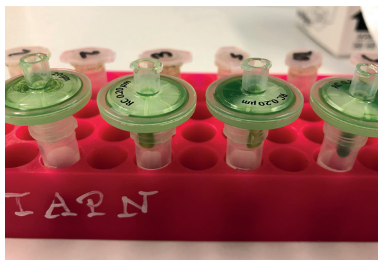
High-performance liquid chromatography (HPLC) measurements were one of the methodologies that Setareh Jamali Jaghdani used in quantification of pigments involved in the xanthophyll cycle. The extracts of the plant's pigments are filtered before the HPLC measurements. (Photo: Jamali Jaghdani)
