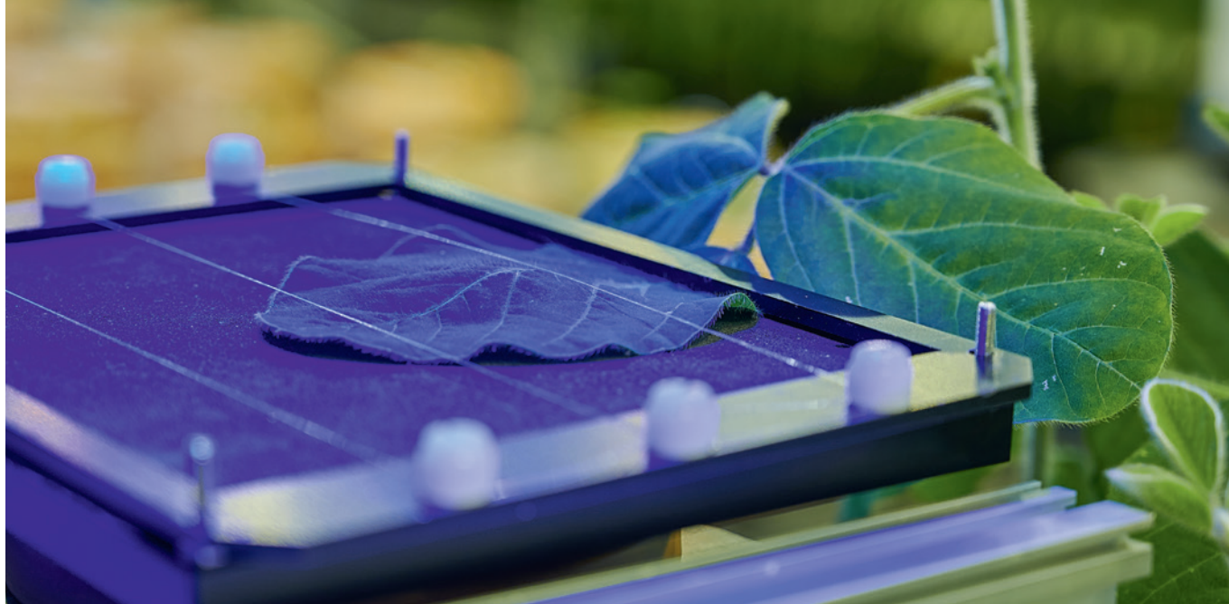
Measurement of chlorophyll fluorescence on a soybean leaf. (Photo: K+S)
