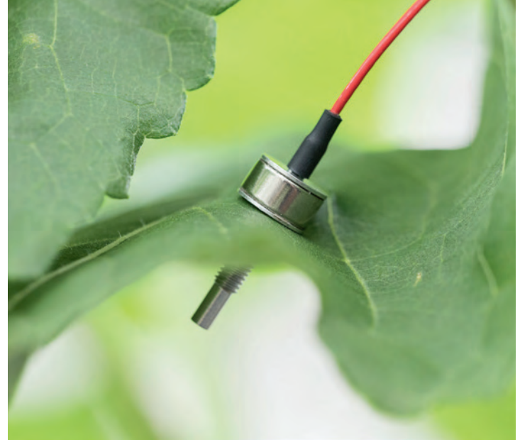
LPCP probe at IAPN: For assessing the plant water status a small patch of a leaf is clamped between two magnets. The force between the magnets applies a constant pressure on the leaf patch. A sensor chip is embedded in the upper magnet and senses the pressure transfer function of the patch - that is the attenuated pressure, P p , in response to the pressure by the magnetic force. Data provided by the chip are continuously monitored and recorded. P p is inversely related to the leaf patch turgor pressure, P c , which relates to the tissue, and ultimately cell-water content. (Photo: D. Jáklí)
