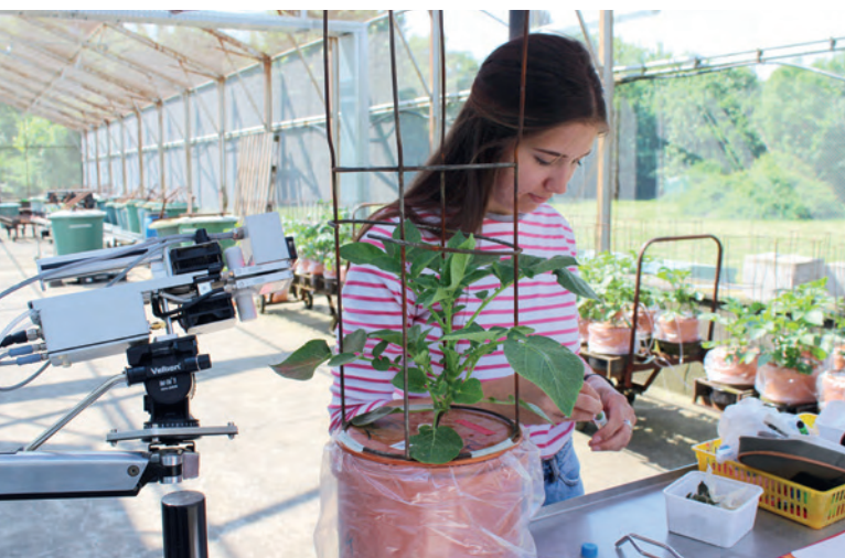
Bachelor's student Henriette Elisabeth Quehl measuring leaf gas exchange (GFS 3000, Walz, Germany) of potato plants that were differently supplied with K and partly exposed to drought stress. (Photos: Tränkner)
