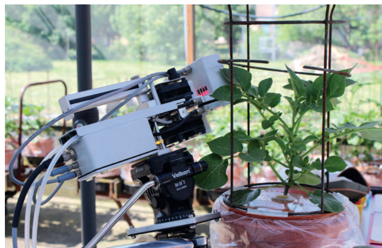
Bachelor's student Henriette Elisabeth Quehl measuring leaf gas exchange (GFS 3000, Walz, Germany) of potato plants that were differently supplied with K and partly exposed to drought stress. (Photos: Tränkner)
