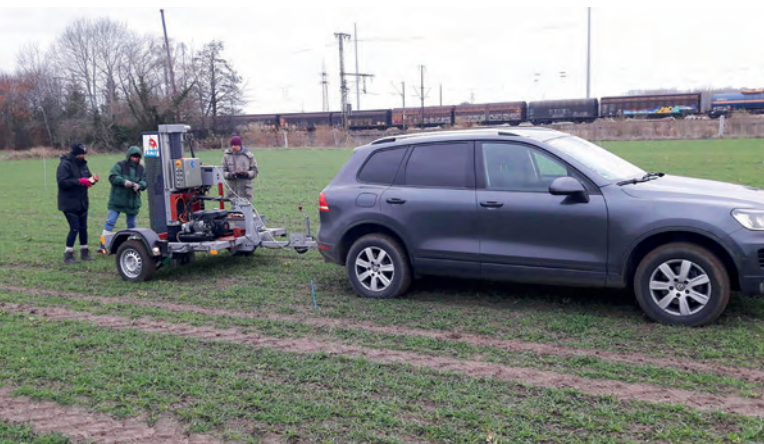
In the course of a new Master project at IAPN soil samples are taken with a hydraulically operated trailer. In contrast to the manual soil sampling, the hydraulic soil sampler allows to obtain easily and fast samples of soil depth up to 90 cm. (Photos: Hanebut)
