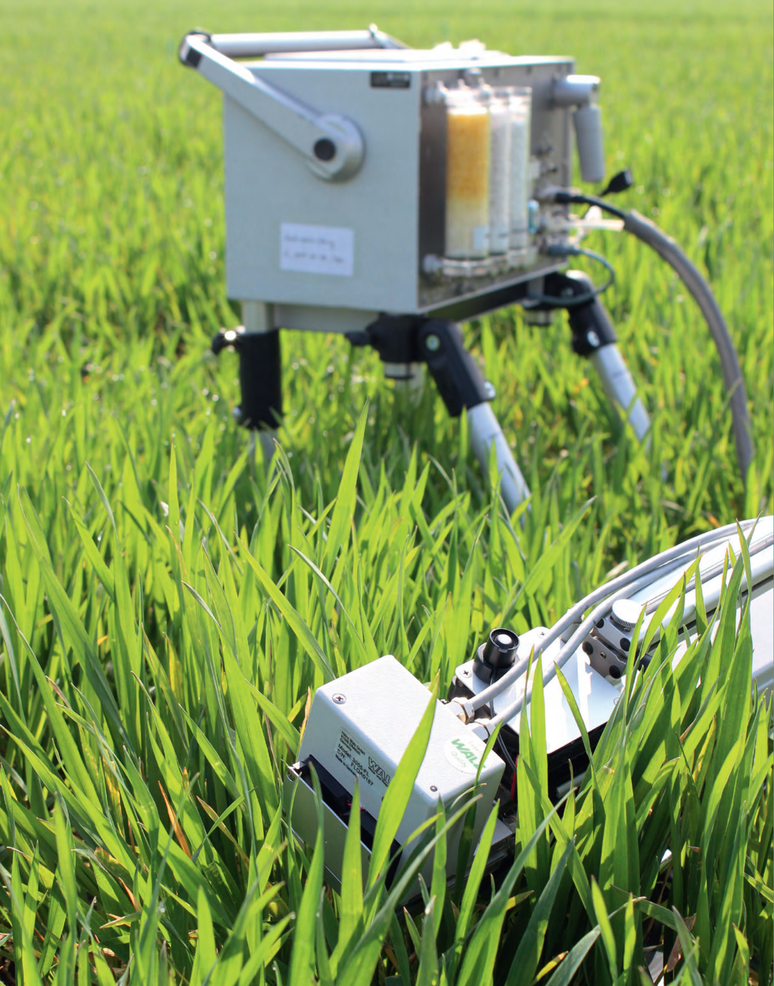
IAPN field trial in Ahlten, conducted on wheat which received different Mg fertilizer treatments. The aim is to study changes in the photosynthetic capacity, pigment composition and water-use efficiency due to different Mg soil concentrations. (Photo: Tränkner)
