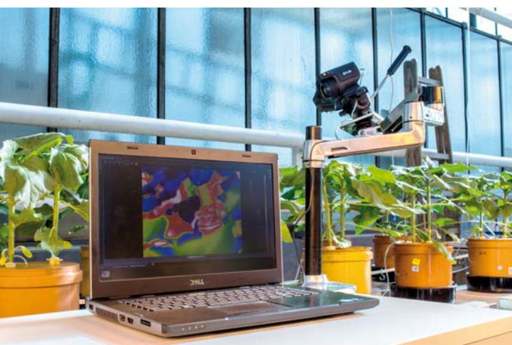
Non-destructive evaluation of sunflower leaf temperature by thermal imaging (T640, FLIR, USA) in the IAPN greenhouse. (Photo: Jákli)
