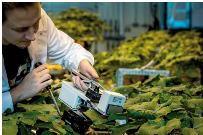
Measurement of leaf gas exchange (GFS 3000, Walz, Germany) of sunflower grown in the IAPN greenhouse. (Photo: Jákli)
