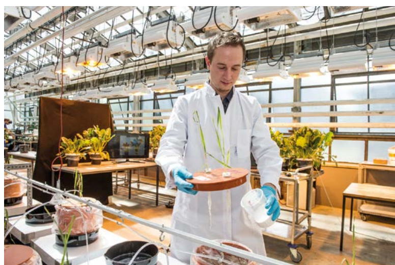
In the IAPN greenhouse, plants are being grown in nutrient solution (left), which allows precise control of nutrients and water. Each pot is positioned on a set of scales, which allows scientists to precisely determine water usage. (Photo: Herwig)
