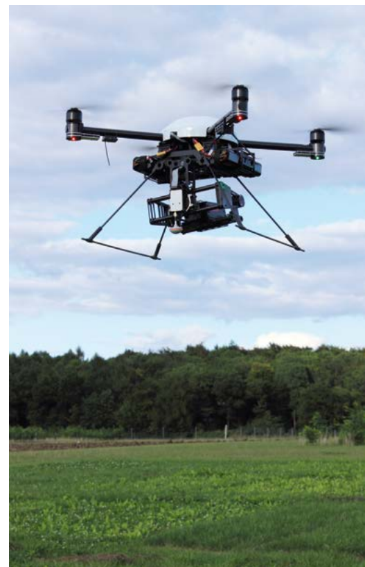
Quadcopter (EagleLive Raptor, EagleLive Systems GmbH, Germany) for remote imaging of crop development and stress tolerance. (Photo: Lingner)
