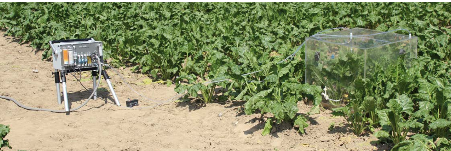
Measuring canopy water use efficiency using a custom-built chamber in combination with the GFS-3000 gas flux analyser (Walz, Germany) of field-grown sugar beet at the SKW Piesteritz experimental site in Cunnersdorf, Saxony. (Photo: Meyer zur Müdehorst)
